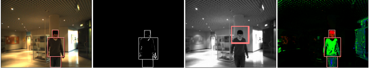
Fig. 2. Video feature maps with the 3-box body model superimposed. From left to right: a) Camera image, b) Foreground segmentation, c) Detector response, d) Color segmentation (head-torso-leg color model projected to the red-green-blue channel respectively).
